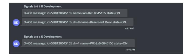
The X-400 device is named WR-8x0 0045155. Rule 2 is executed when the device enters/exits alarm state and replaces the {name} variable with the device name.
