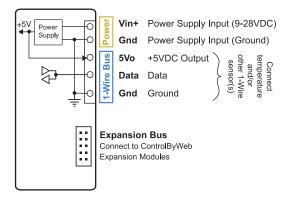
**Warning:** The maximum number of attached expansion modules is determined by power supply voltage and current, and type of modules attached. For some installations, additional power supplies and expansion bus power injectors may be required.
